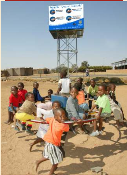
PlayPumps International – an organization that helps build water wells in Africa, with a system whereby children playing on merry-go-round equipment provide energy to pump up and store water from a well.
