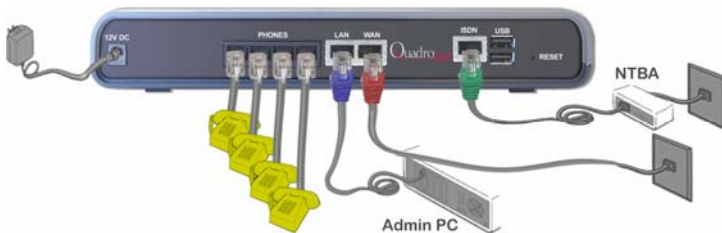
Fig. I-14: Installation: Quadro4xi used as an Internet Access Router
