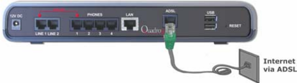
Fig. I-15: Installation: Quadro4xa used as Internet Access Router
