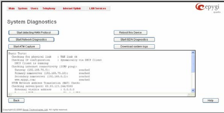
Fig. I-58: System Diagnostics - Network Diagnostics page
