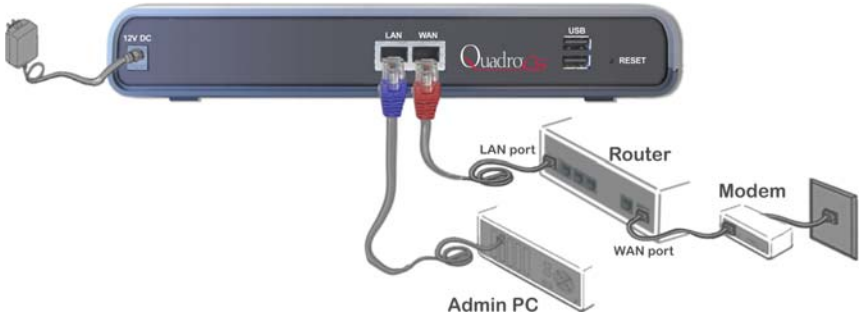
Fig. I-5: Installation: QuadroCS behind a router
